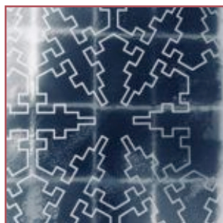
Satellite sandwich with fractal antenna metamaterial over solar cells. (Courtesy © Fractal Antenna Systems, Inc.)
